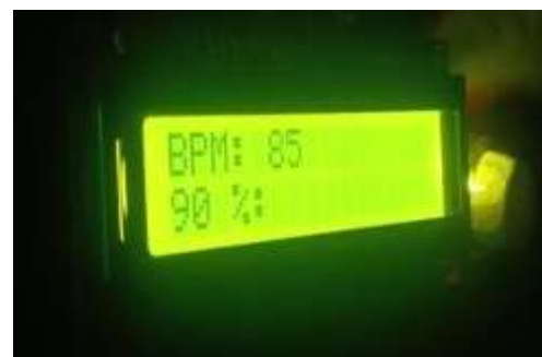
Figure 8: Results of BPM and SpO2 sensor
