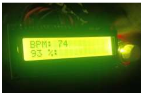
Figure 8: Results of BPM and SpO2 sensor
