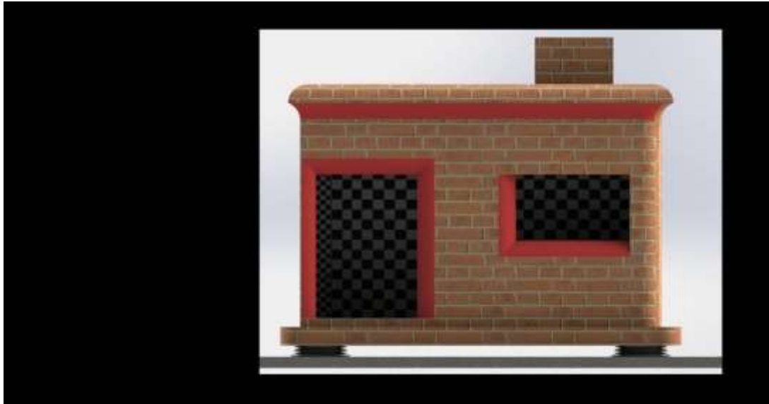
Figure -1, (A house which is designed with Base Isolation method, which is help to protect the building by the affect of earthquake .This image is designed in Solid Works software , elastomers rubber bearings)
