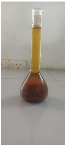
Fig.12 e-waste and NaOH are Combined in the ratio 1:6
