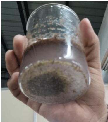
Fig.17 Sink and Float method for separation of metals and plastic particles
