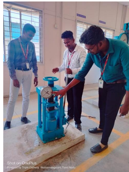
Fig 6 : Compressive strength on plastic pavement block
