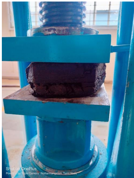
Fig 6 : Compressive strength on plastic pavement block
