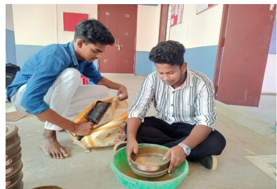
Fig 2: sand sieving process
