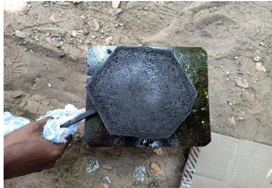
Fig 5: Allow the pavement block to cool and cure at room temperature
