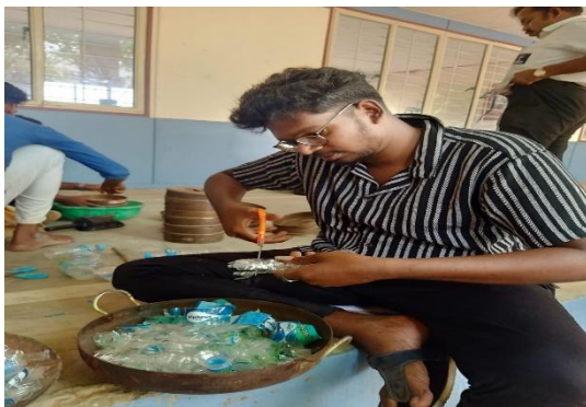
Fig 1: cutting the plastic into small pieces
