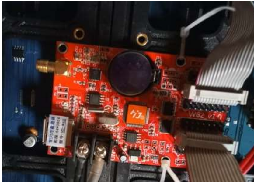
Fig 3.2: Controller Unit of the Digital Display System
