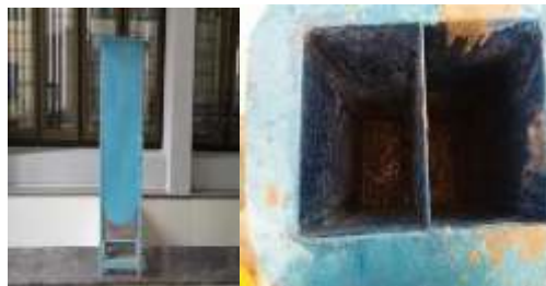
Fig 5: U- Box Test
