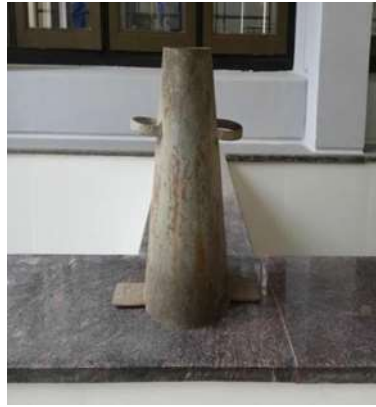
Fig 2: Slump Cone test
