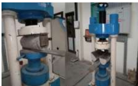
Fig 6: Compression Test On Cube
