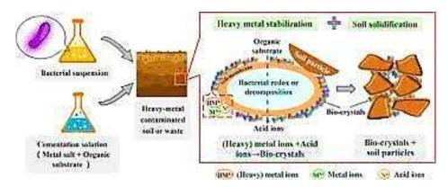
The cementation process not only improves the mechanical properties of the soil, such as strength and stiffness, but also enhances its durability and resistance to erosion. Furthermore, the formation of calcium carbonate within the soil pore spaces creates a cementing matrix that helps stabilize the soil structure and prevent settlement.
