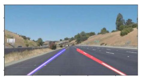
Even the slowest processing speed measured at 11 frames per second remains ample for accurate lane-line detection. A frame rate of 10 frames per second is deemed sufficient for the intended application, highlighting LaneRTD's suitability for real-world deployment.
