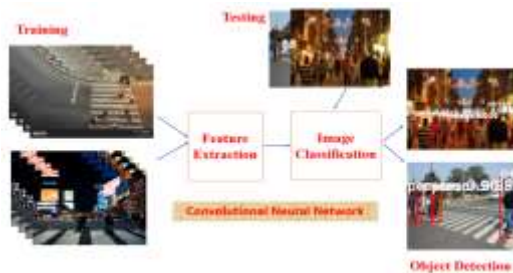
Fig.1. Block schematic for the object detection system.
