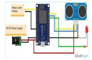
It describes the water flow system by giving the water flow and detecting overflow. It also uses an observational method to detect faults in sewer pipe blocks based on water flow. A smartdrainage system has sensors that detect blockages and floods. The Node MCU Wi-Fi module is the user interface of the Wi-Fi organization to import or transfer data to the network. The center of the Wi-Fi module sends this information in its entirety to the database.
