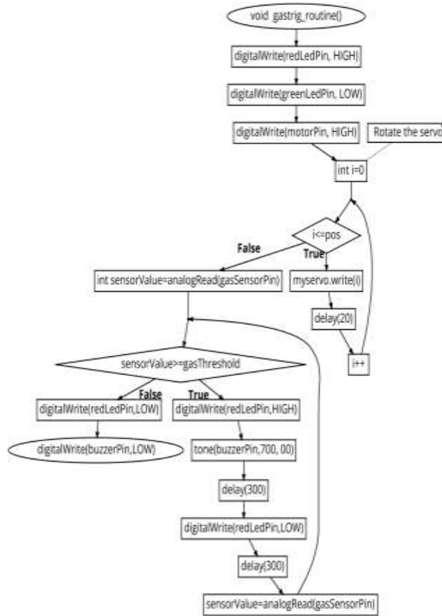
Fig. 8 – Gas trigger routine loop of the automatic ventilation system.
