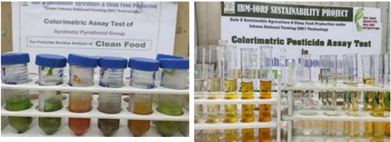
Fig 20 : Pesticide residue analysis of vegetable samples through colorimetric assay test under ‘Clean Food’ Program
