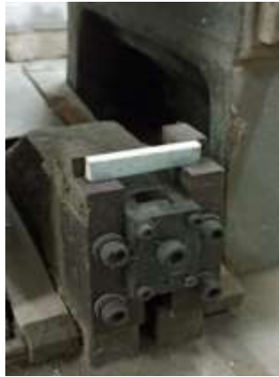
Fig.2.6 (a). Impact Test Machine, (b). Specimen fixed on testing machine
