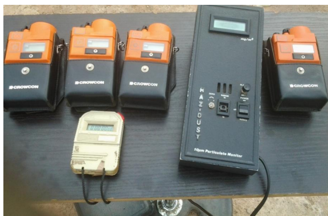
Plate 1. Crowcon Gasman Monitors used in the Study (Photo by Jenny & Natty W, 2022)
