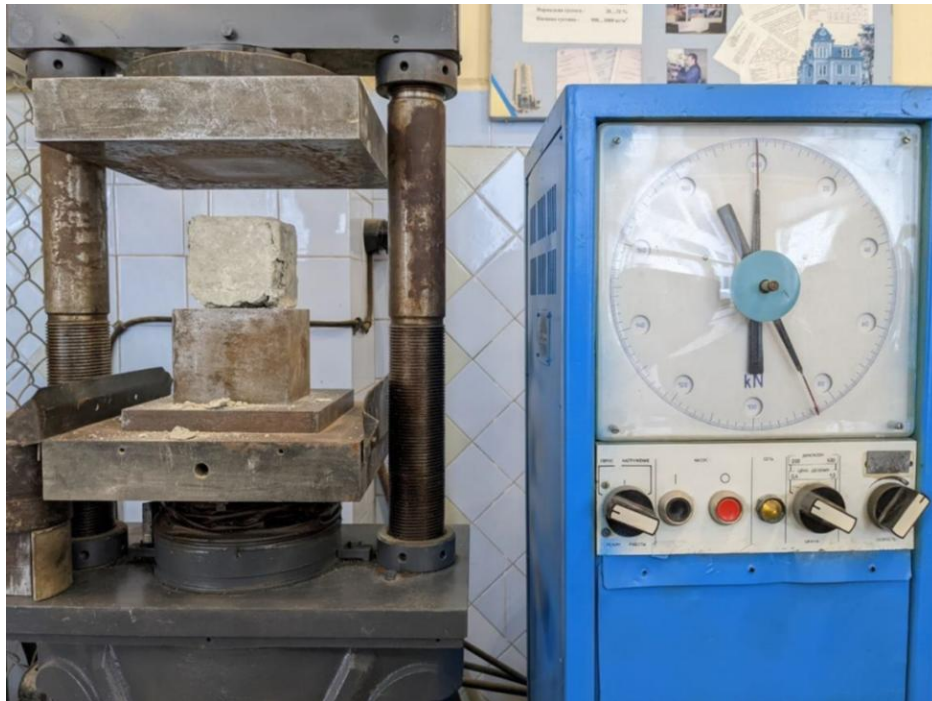
Fig. 3. Compressive strength tests of concrete samples after being in the biocompartment.
