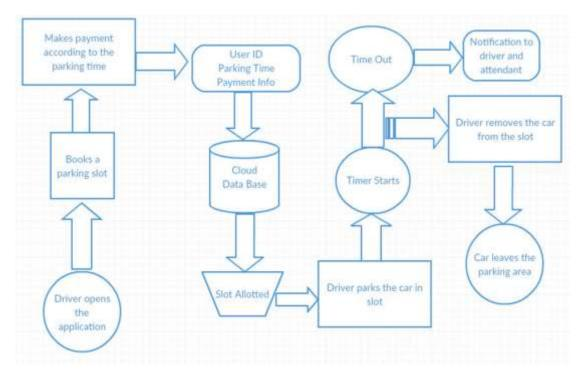
The above figure depicts the working of the system at every stage for checking the availability of parking space to actually park a car in a vacant parking slot. The smart parking system can be implemented in the parking area of a shopping mall. The steps that the user needs to follow to use the parking system is given below.
