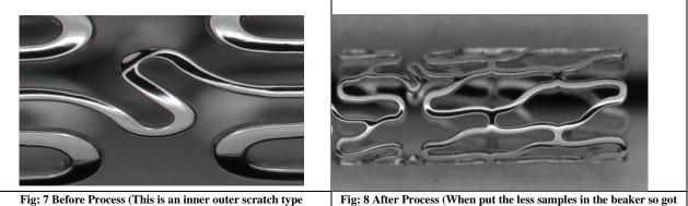
Fig: 7 Before Process (This is an inner outer scratch type rejection this type of rejection has occurred during descaling process when more samples are put in the beaker)
