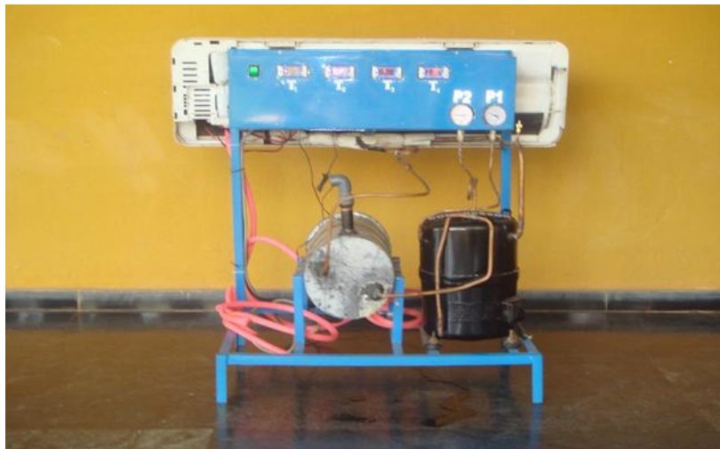
Fig.3: Experimental Set up of Heat pump
