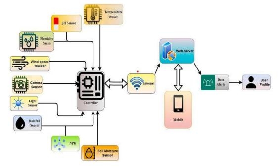
1.LDR (Light Dependent Resistor): This sensor is sensitive to light intensity. Its resistance decreases with increasing light levels, and hence, it is used in applications such as automatic lighting systems and sunlight monitoring.
