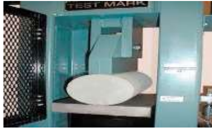
Fig.15. Compression test equipment for evaluating split tensile capacity
