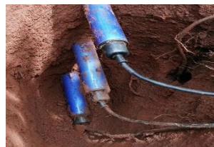
Figure 2 MP406 soil moisture
