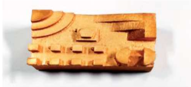
Fig 14: EDM electrode Fabricated by RP [14]
