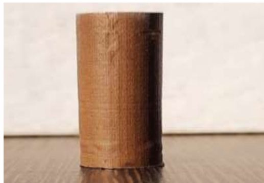
Fig 16 : EDM tool developed by ADAM process [17]
