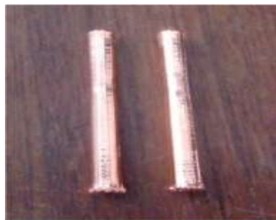
Fig 10: Metalized FDM electrodes [1]
