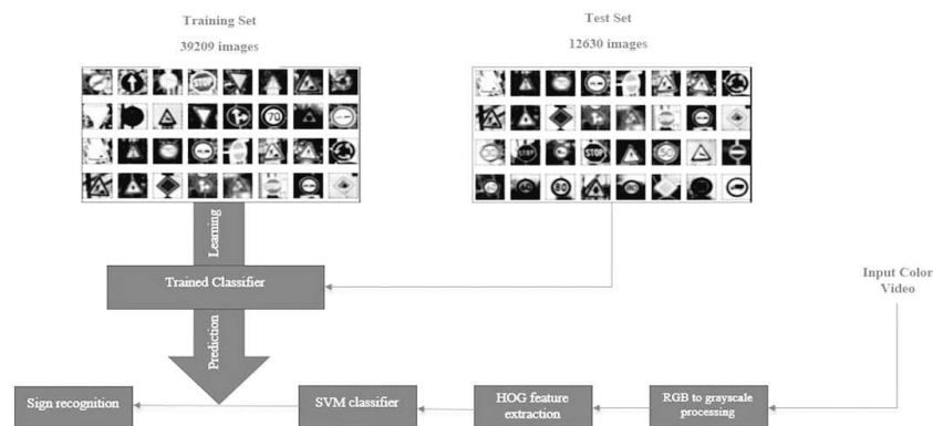
Fig.3.4: Road Sign Detection and Classification Architecture Using LeNet CNN [13]
