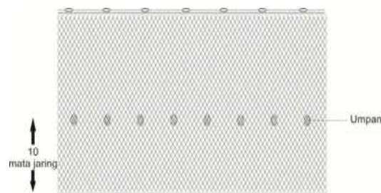
Fig 1 - Placement of Bait on the Bottom Set Gill Net
