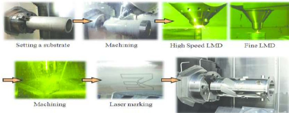
Fig.6. Application example for hybrid process
