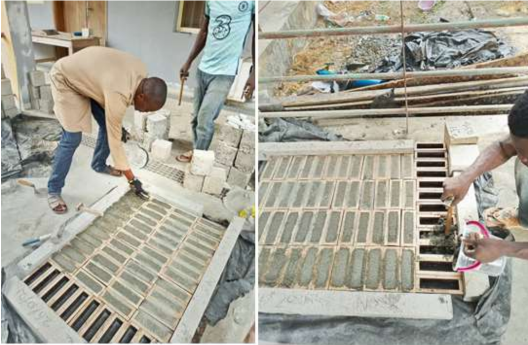
Figure 2: Sample preparation of mortar beams
