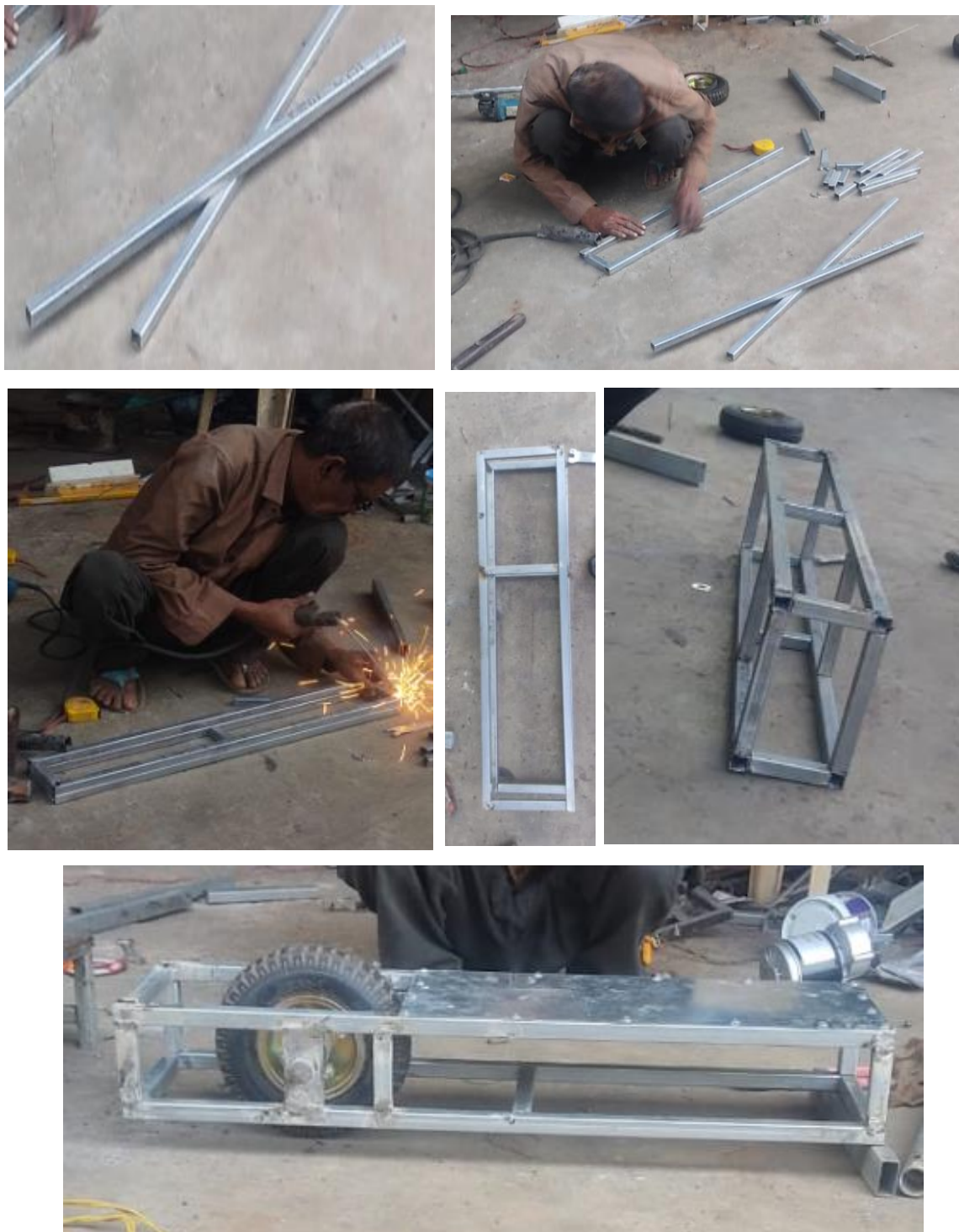
FIGURE 18. Structural Hardware Development for E-Scooter Frame
