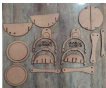
Fig. 6 - Total components cut by using CO 2 laser cutting
