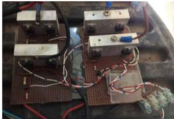
Figure 6 Construction/Soldering of H-bridge Driver Circuit
