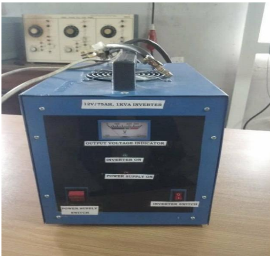
Plate 6a: Front view of an inverter
