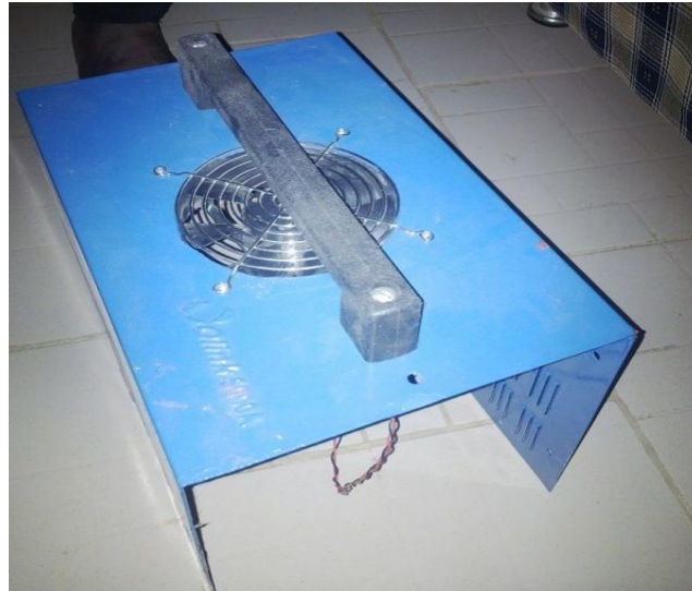
Plate 5: A diagram showing the constructed inverter casing
