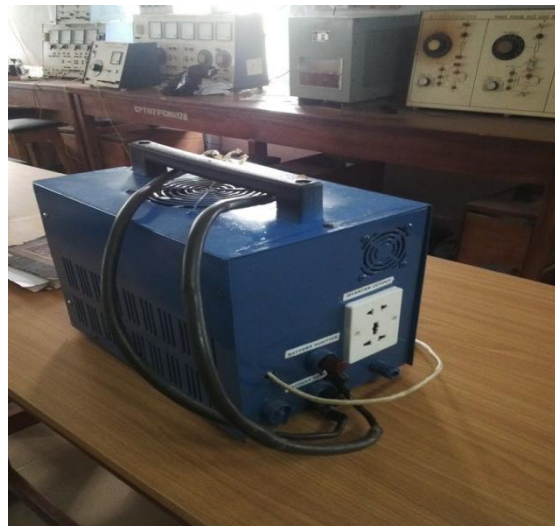
Plate 6b: Back view of an inverter
