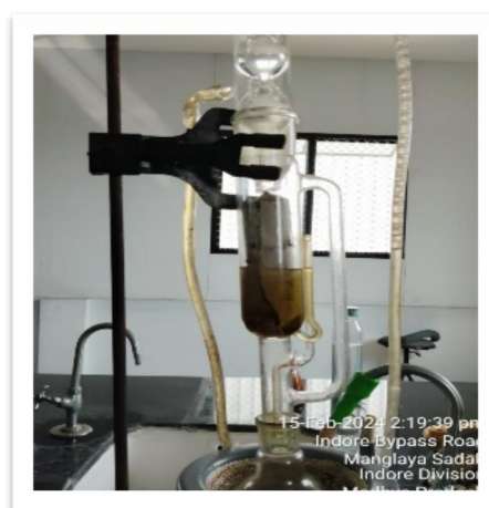
Figure No: 7 Soxhlet Extraction Process
