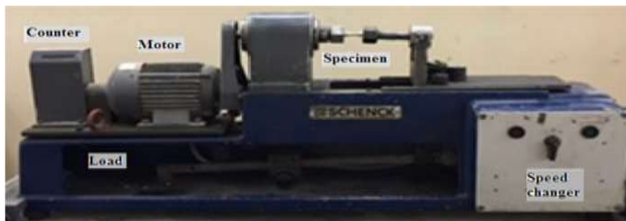
Figure 2. Fatigue test setup
