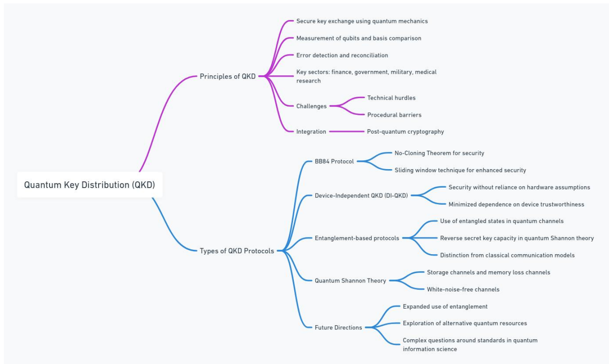
Figure 3: The principles and types of Quantum Key Distribution (QKD)
