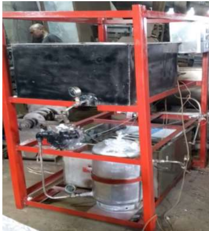
Plate 1 Pictorial View of the Mini –OTEC Plant
