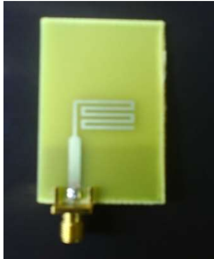
Fig 6- Fabrication of Monopole antenna
