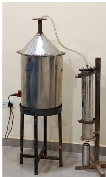
Fig. 3: Fabricated Extractor (Distiller)
