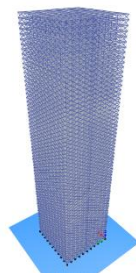
Fig. 2 A perspective view of the Diagrid structure
