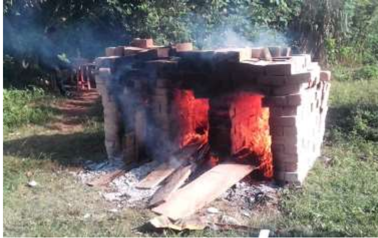
Fig 3 - Firing of insulating bricks
