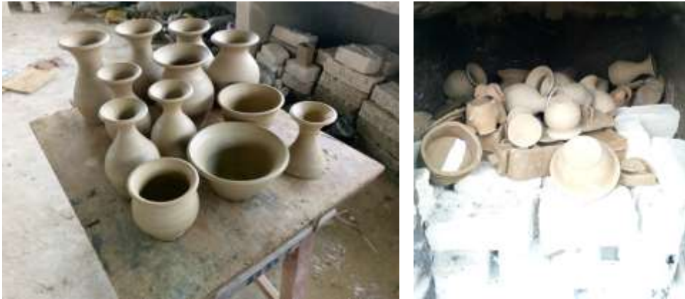
Fig.8 - Wares ready for firing; Loading of bricks and wares
