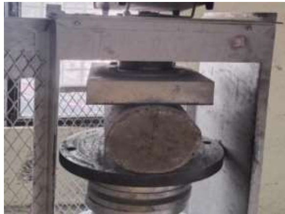
Fig. 8 Split Tensile Strength Test Setup
