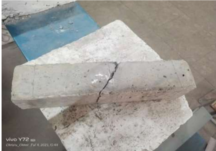
Fig. 11 Flexural Strength Test – Failure Beam
