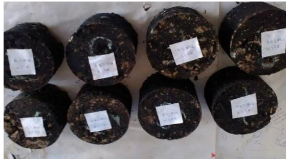
Fig. 3 – Shows Marshal Test Samples.
