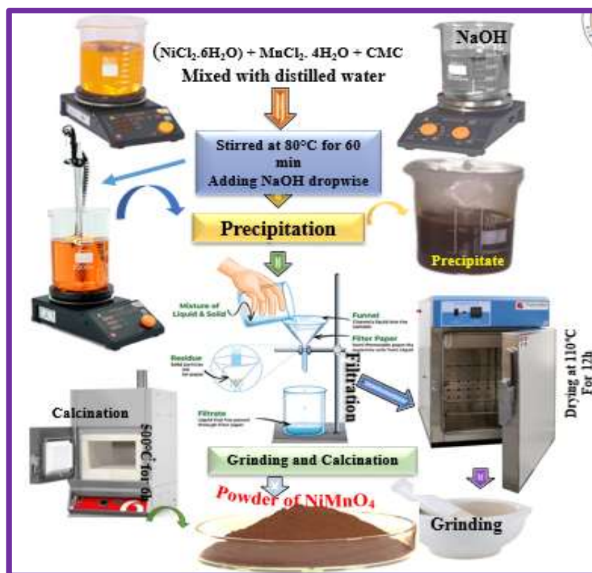
Figure 1: Synthesis of NiMn 2 O 4 nanoparticles by Co-precipitation method.
