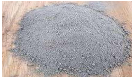
Figure 3: Ordinary Portland cement
