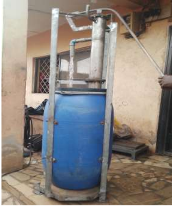
Fig. 1. Diagram showing the fabricated simplified reciprocating water pump
