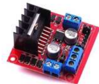
Fig (4). L298 Motor Driver
