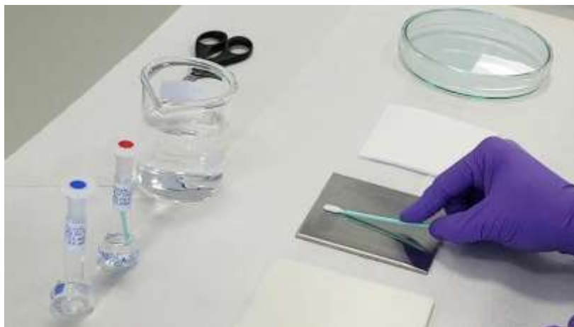
Fig. 4. Swab Sampling Technique
