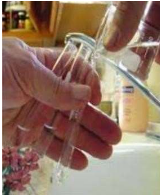
Fig. 5. Rinse Sampling Technique
