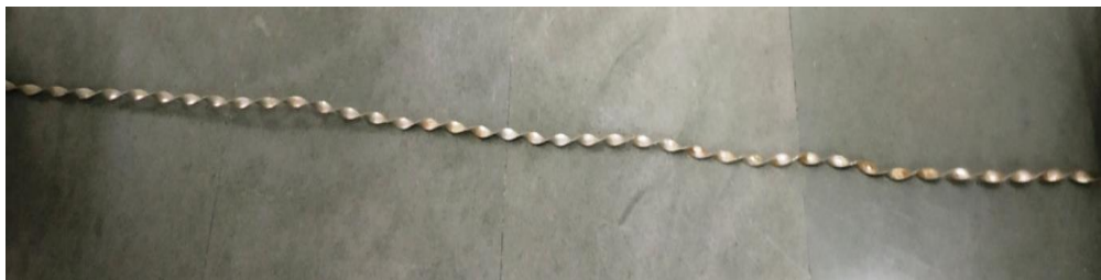
Figure 1 full length twisted tape
