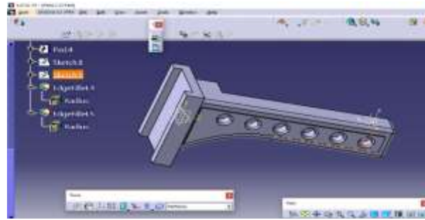
Fig. 3 – Apply edge fillets to remove sharp edges
