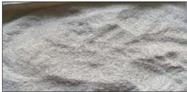
Figure Obtained RHA grain size of 3.8µm (Stage-IV)
