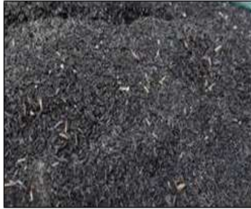
Figure Rice husk was converted into ash by open burning method at a temperature ranging from 300°C to 450°C
