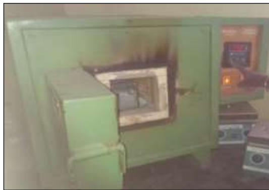
Figure Fired husk residue ash was further burnt at a temperature of 650°C over a period of 2 h (Stage-III)
