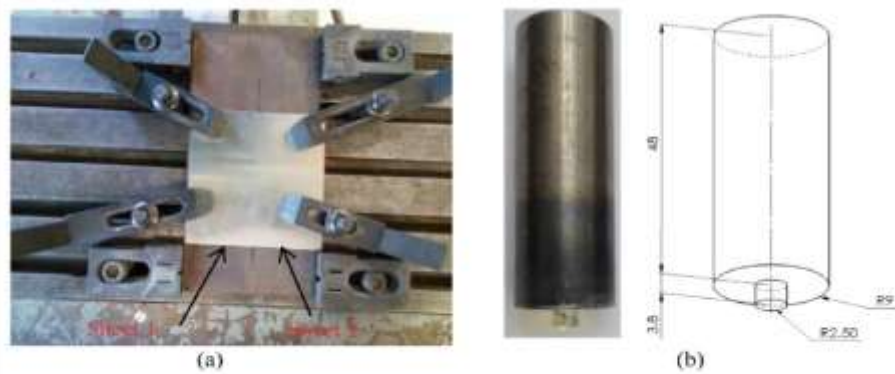
Fig. 1. (a) Clamping system, (b) Welding tool (unit: mm).
