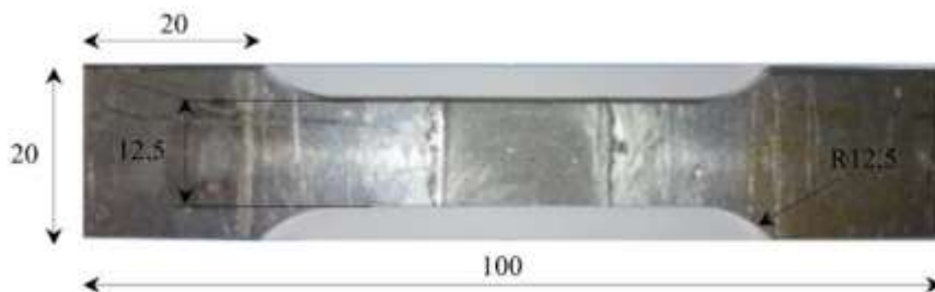
Fig. 3. The tensile test specimen (unit: mm).
