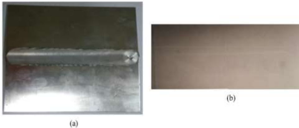
Fig. 4. (a) Friction-stir weld in 2024-T3 aluminum alloy, (b) X-ray image of the weld.
