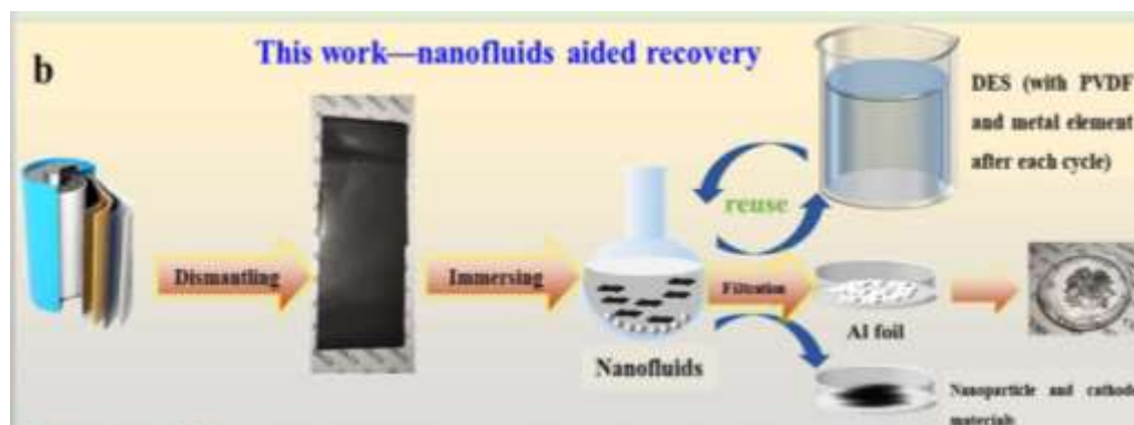
Fig-1: Flow diagram of eutectic solvent based nanofluids.
